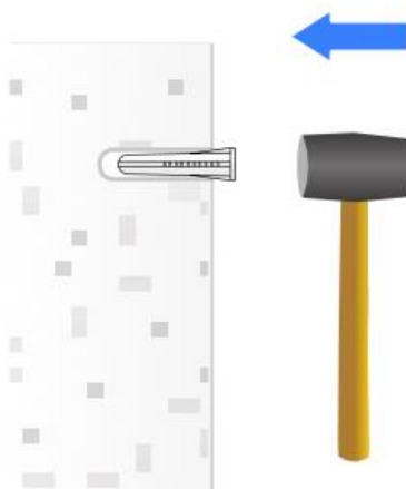
Figura 1-6 Martele as buchas de parafuso
